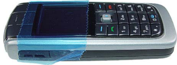
2.) Protect the Window with a protective film.
