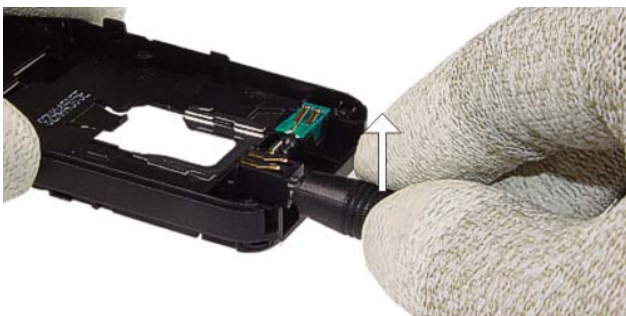
15.) Remove the DC-Jack with a DC-Plug .
