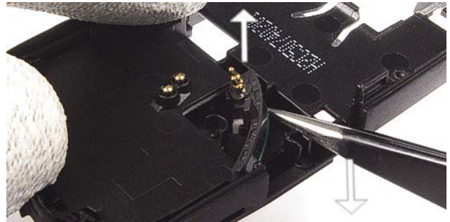
20.) Remove the Bluetooth Antenna with tweezers.
