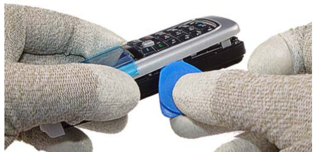
4.) Unlock the side snaps with SRT-6 when opening the A-Cover.
