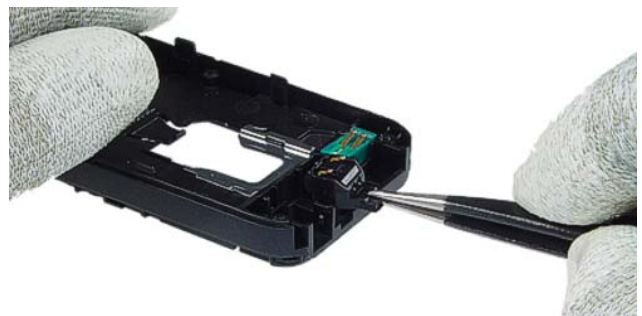
16.) Remove the Microphone with tweezers.
