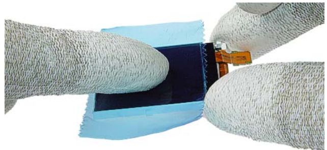
12.) Protect the LCD Module with a protective film.
