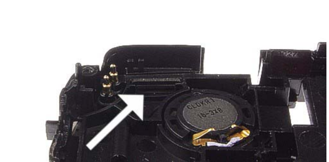
22.) Note, that the IHF Net stays in place during disassembly.
